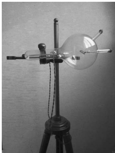
Fig. 2.1 An early gas (ion) X-ray tube mounted on a wooden stand.
