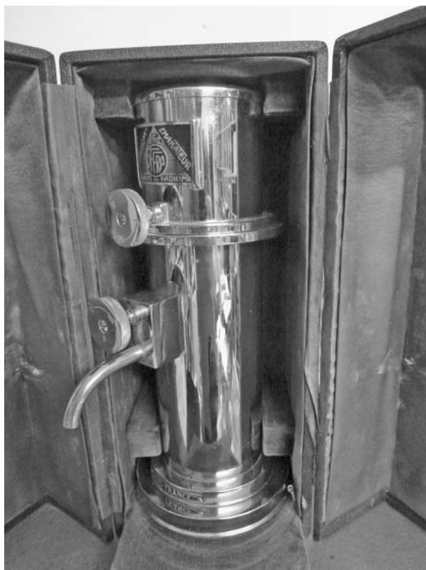
Fig. 12.3 The infamous 'Radium-Émanateur' from 1935 used for producing radioactive drinking water.
